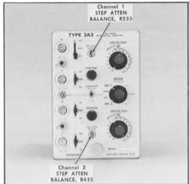
Fig. 6-3. Location of channel 1 STEP ATTEN BALANCE control, R235 and channel 2 STEP ATTEN BALANCE control, R435.
